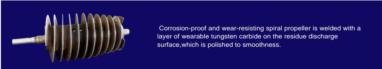
Corrosion-proof and wear-resisting spiral propeller is welded with a layer of wearable tungsten carbide on the residue discharge surface, which is polished to smoothness.
